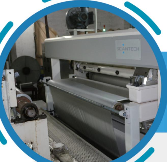
在线测厚仪 On-line thickness gauge measuring
