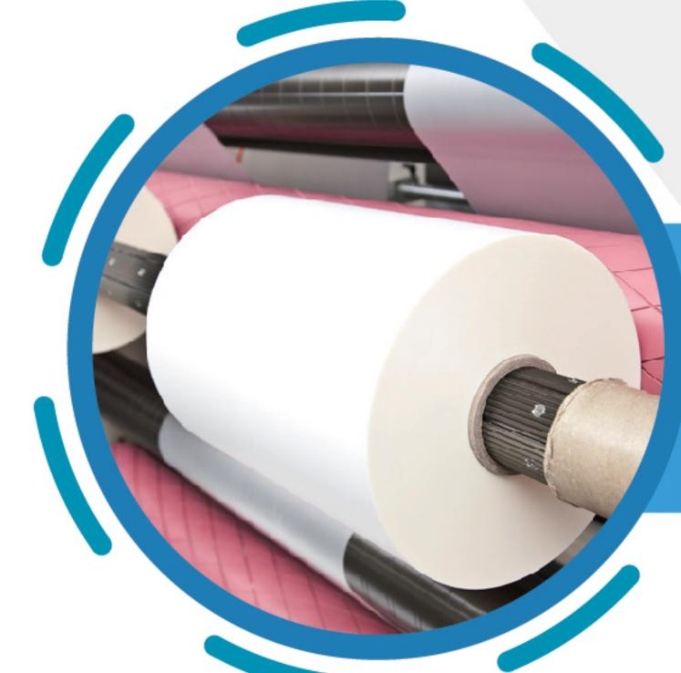
分切,检验收卷松紧,端面平整度 Slitting into different size, Rewinding in smooth roll
